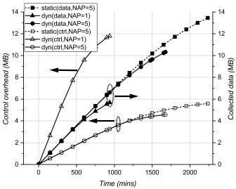
Fig. 6. Pseudo-dynamic vs. static SD-WSN accumulated control overhead and collected data.
