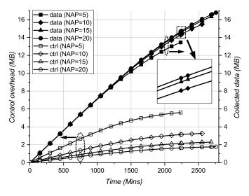
Fig. 2. Accumulated control overhead vs. accumulated collected data for large SD-WSN.
