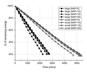
Fig. 3. Remaining energy of large vs. small SD-WSN over simulation time.
